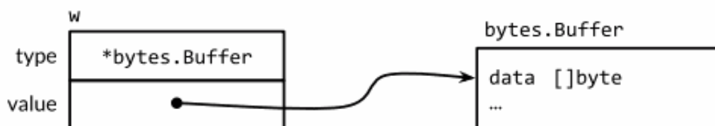
Figure 7.3. An interface value containing a *bytes.Buffer pointer.
