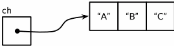
Figure 8.3. A full buffered channel.
