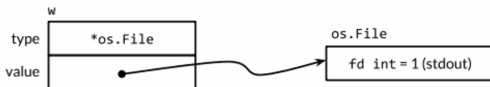
Figure 7.2. An interface value containing an *os.File pointer.
